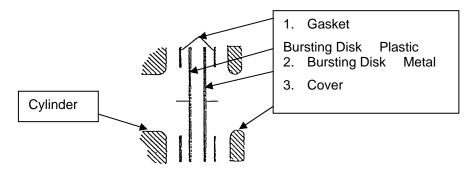
Before refitting ensure the radiused edges of the cylinder hole and cover are smooth and have no burrs or corrosion.
