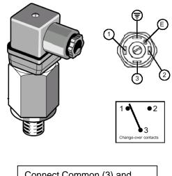
Connect Common (3) and Normally Open (2) terminals to compressor control panel
