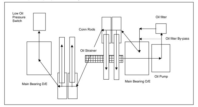
An oil pressure gauge indicates if over-pressure and is relieved through a safety valve within the oil pump. A protective Low Oil Pressure Switch or LOP is installed to shut-down the compressor if the pressure falls below 1 bar (15 psig). On starting if the oil pressure has not built up within about 10 seconds the LOP, connected to a delay timer in the motor starter control, will shut down the compressor.
