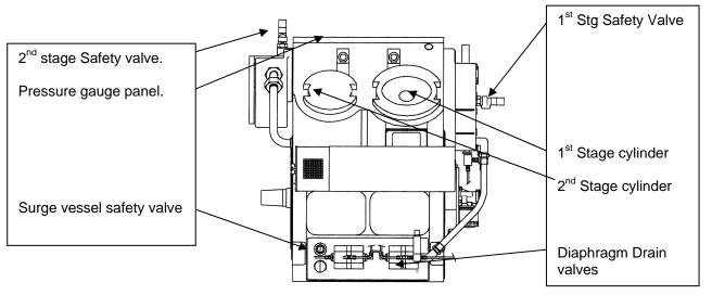
The R - 5437.1.IA compressor is a reciprocating 90° vee configuration, 4 stage, single acting, water cooled machine with the 1st and 3rd stage lines on one crank throw, and the 2nd and 4th stage lines on the opposite crank throw of a counterbalanced crankshaft. The running gear consists of the crankshaft, bearings, connecting rods, oil pump, cylinder lubricator and other accessories.
