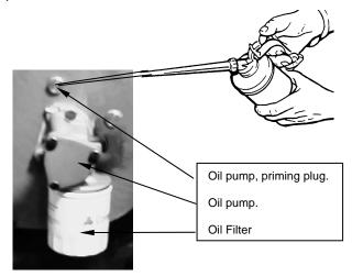
Remove oil pump priming plug, using pump type oilcan, prime system with correct grade oil. Replace plug. Arrange for compressor to discharge temporarily to atmosphere (unloaded) by opening the manual drain valve at the 4<sup>th</sup> stage coalescer filter drain and electrically disconnect solenoid valve by removing cable plug from solenoid coil.
